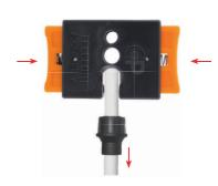
Expose centre dielectric by bearing back the sheath and shield.
