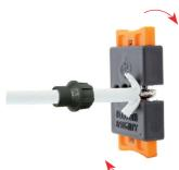
Push the exposed copper core into the F female connector, slide the sheath and shield over the thread and slide the CaP to the start of the F connector.
